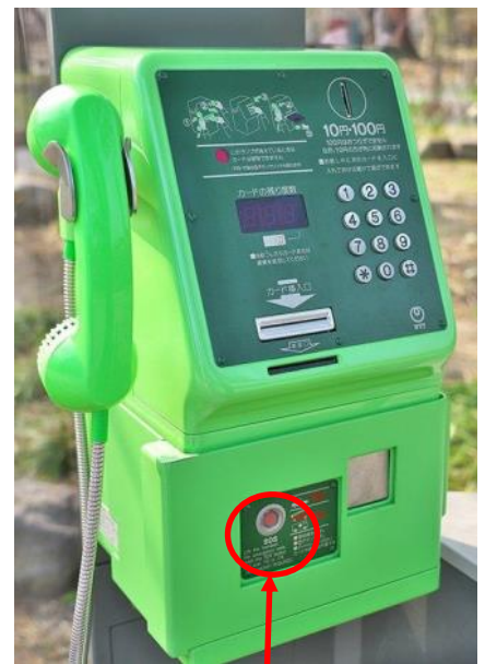
Emergency notification button
